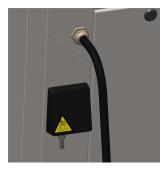
Figure 8: Hose connection for compressed air
