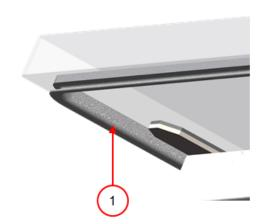
Figure 28: Replacing the Lid Gasket
