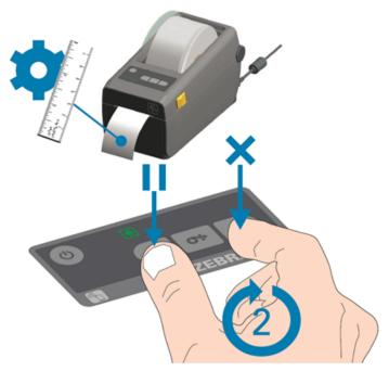
Figure 19: Aligning the Printer
